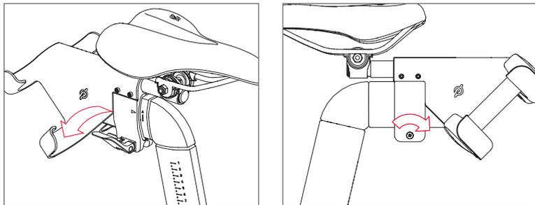
**⚠ WARNING:** Do not over-tighten the seat slider adjustment knob. Over-tightening could result in malfunction or breakage.
